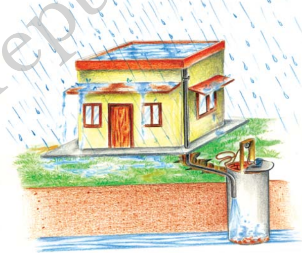
(b) Recharge through Abandoned Dugwell
